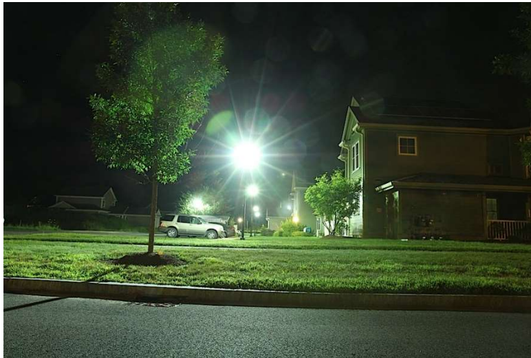
Figure 2: Example of glare from a light pole
