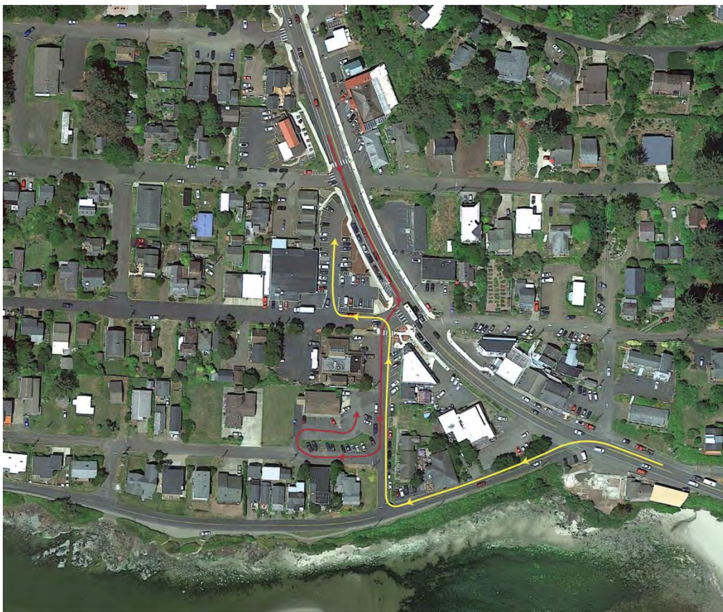
Figure 9: Possible problematic circulation patterns for southbound traffic (red) and northbound traffic (yellow) searching for parking
