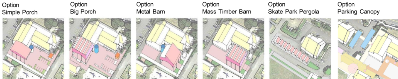
Caption: Six candidate options were considered to boost collection capacity to generate as much power as would be required to sustain the Southedge activities for up to 3 months when power generation is at its lowest.
