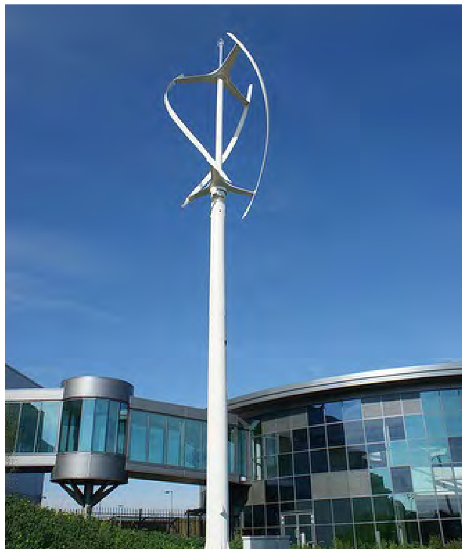
50 kW vertical axis wind turbine (Quiet Revolution, UK)
